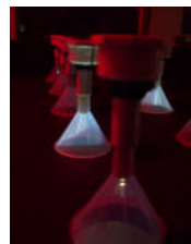
(B) Close-up of poles in the Brown and Wintersteen apparatus. Pole in foreground is not illuminated. Two poles in background are illuminated. Pole illumination was used as a cue indicating whether pole had been visited earlier during the trial.
