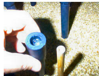
Figure 8. Outer sleeve of pole (being held) and inner core (to right). Sham pellet (on every pole) is placed in well at top of inner core. Baited poles have a second (accessible) pellet in the well at top of sleeve.
