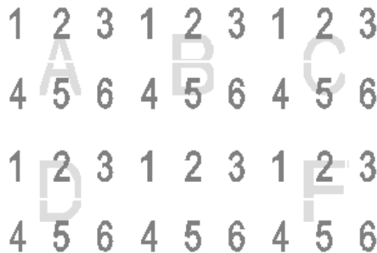
Figure E3. Region division. The obstacle that occupies places 2 and 5 divides the region in two subregions E and E'.
